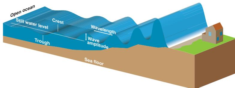
Figure 2: Change in wave length and height as a tsunami approaches the shore
